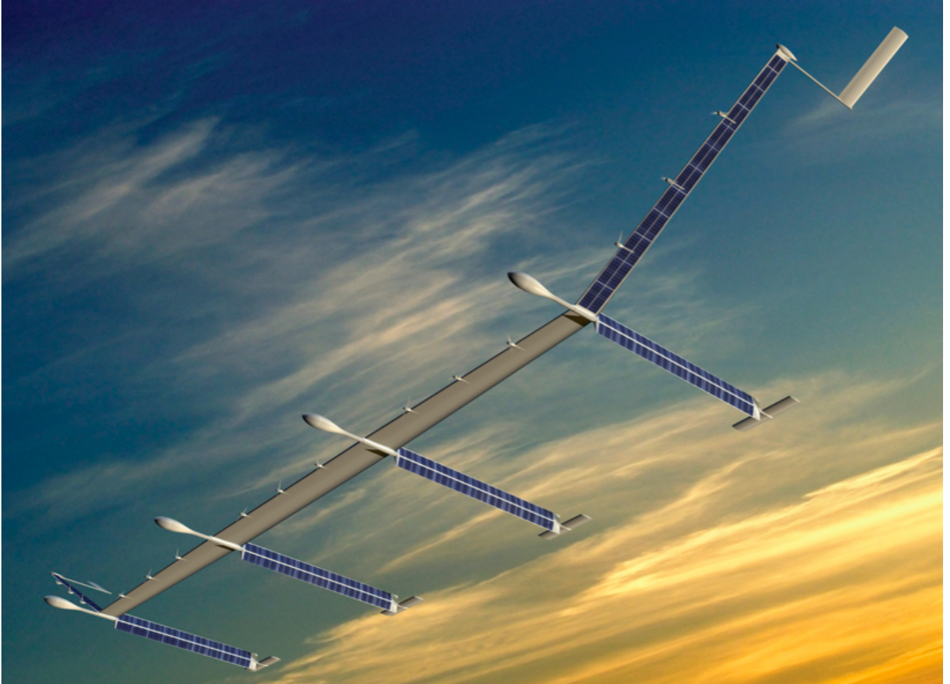
A portrait of the Boeing SolarEagle (Vulture II), a High Altitude, Long Endurance (HALE) unmanned aerial vehicle solar-electric spy plane developed by Boeing Phantom Works.
