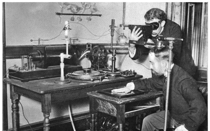
Taking an X-ray image with early Crookes tube apparatus, late 1800s. License: public domain.
