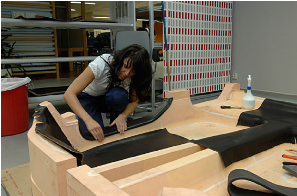
At work on the Volvo production floor lining the XC60 concept car in dark-brown saddle-quality leather. © Volvo Car Corporation
