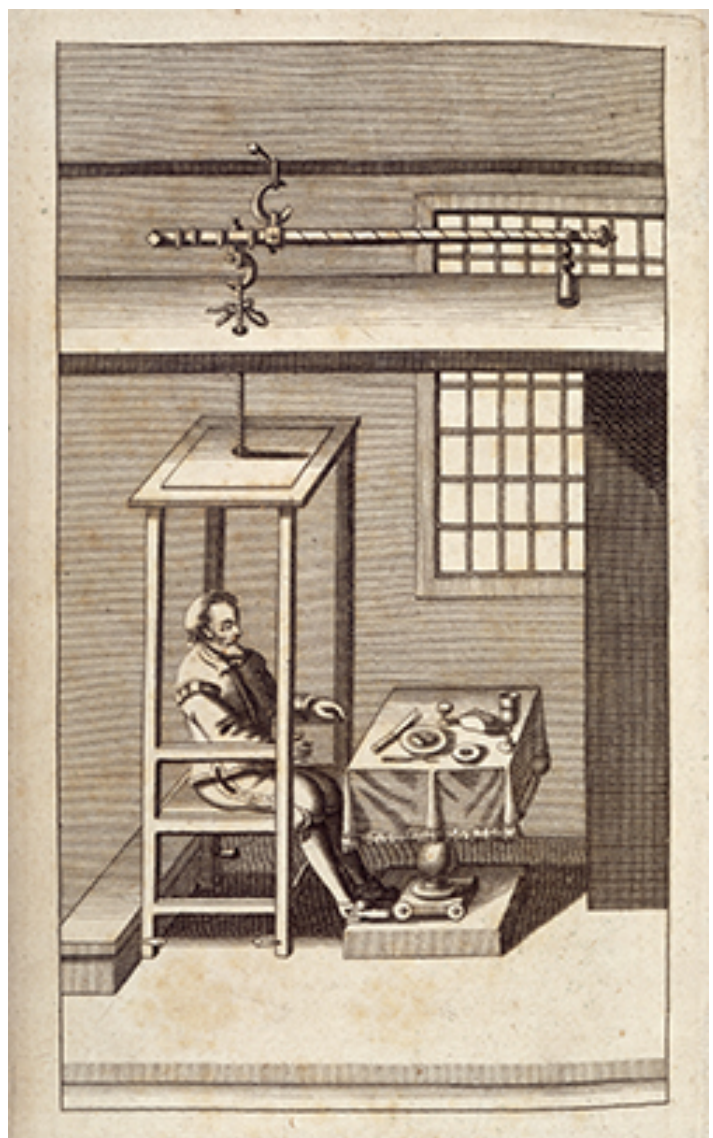
Santorio sitting in the balance that he made to calculate his net weight change over time after the intake and excretion of food stuffs and fluids. Photo: CC BY 4.0, via Wikimedia Commons/Wellcome Collection.
