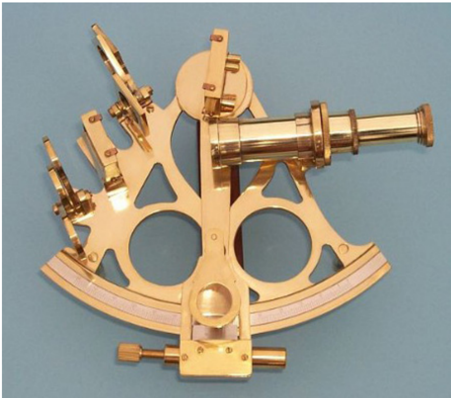
The sextant, a nautical instrument which determined the angle between a celestial object and the horizon.
