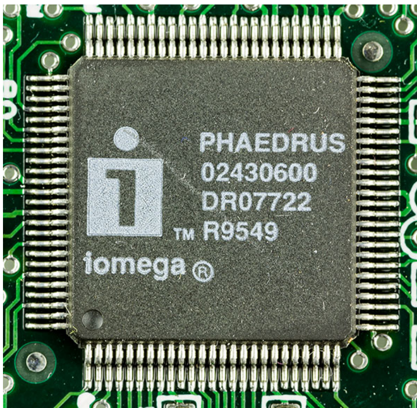
Iomega Phaedrus microchip used on mainboard of Iomega ZIP-100, parallel port printer pass-through.
